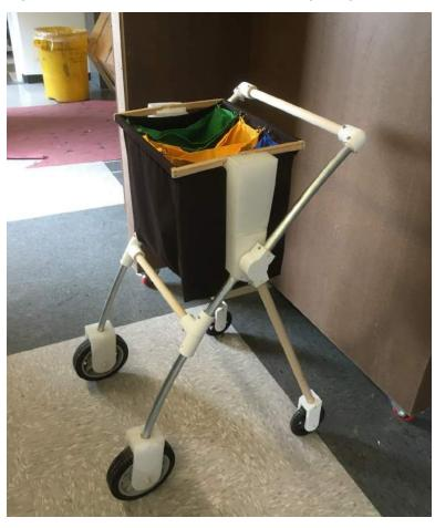
bars were made of wood sticks. They were connected together by screws and A/B glue was also used in some joints to enhance the strength. It could hold the basket
