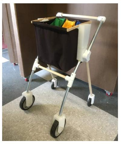
with groceries, but not rigid enough for a person to put his weight on the handle bar, since the 3D printed joints were easy to break apart.
